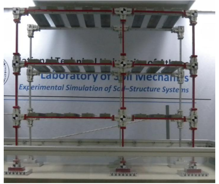
Figure 3. Photo of the reduced-scale ( N = 10 ) physical model.
